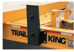
**Bolt-on Spare Tire Carrier** Optional feature that allows you to safely mount and easily remove a spare tire.
