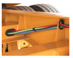
**Protected Electrical System** Features rubber-mounted, shock-proof, sealed lights and rubber grommets for all wiring through the frame for longer, troublefree, low-maintenance performance life.
