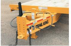
**Adjustable Hitch** Accommodate a wide variety of towing vehicles with an adjustable 4-bolt hitch rated for the full GVWR of the trailer.
