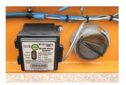
**Break-Away System** Sealed electric break-away system on TK20/24 models with electric brakes located in tongue area.
