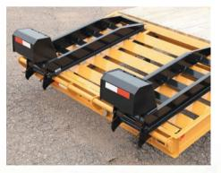
**Spring-Assist Ramps** Standard self-supporting 5 foot raps with spring-assist are lightweight, strong and easy to handle. Choose between standard ladder-type or optional wood-filled or air-assist ramps.
